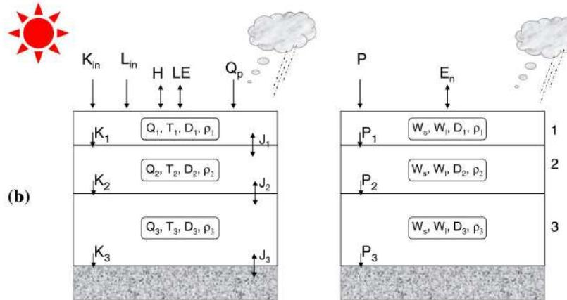
**K<sub>in</sub>** (short wave radiation), **L<sub>in</sub>** (longwave radiation), **H** (sensible heat flux), **LE** (latent heat flux), **J** (conduction heat flux), **Q** (snow layer heat content), **Q<sub>p</sub>** (advectional heat from rain and snow), **W** (snow layer SWE), **W<sub>l</sub>** (snow layer liquid water content), **D** (snow layer depth), **p** (snow layer density), **P** (precipitation), **E<sub>n</sub>** (evaporation)
