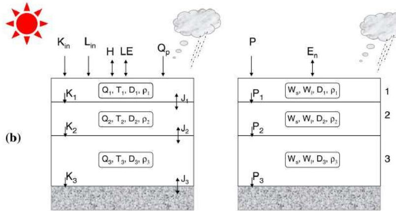
$K_{in}$  (short wave radiation),  $L_{in}$  (longwave radiation),  $H$  (sensible heat flux),  $LE$  (latent heat flux),  $J$  (conduction heat flux),  $Q$  (snow layer heat content),  $Q_p$  (advectional heat from rain and snow),  $W$  (snow layer SWE),  $W_l$  (snow layer liquid water content),  $D$  (snow layer depth),  $\rho$  (snow layer density),  $P$  (precipitation),  $E_n$  (evaporation)
